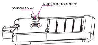
Insert the photocell socket into the opening.
