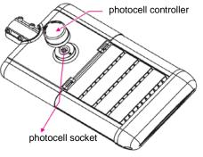
Use screw driver to remove securing bolts (or press down the spring snaps at two sides, if applicable) and open the driver compartment cover.
